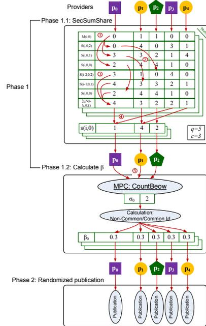
Fig. 3: An example of  $\epsilon$ -PPI construction algorithm
