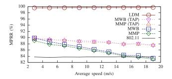
Figure 5. Multicast packet reception ratio for each protocol.
