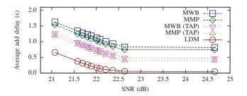
Figure 3. Add delay for each protocol under different SNR.
