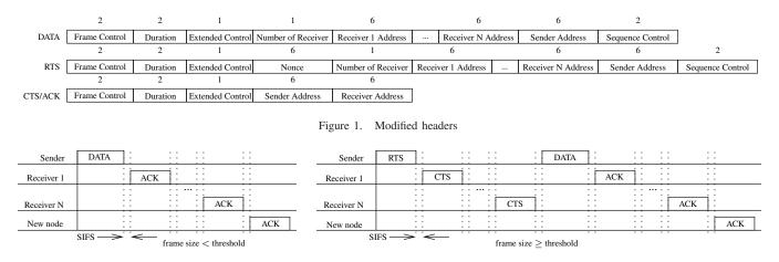
Figure 2. Link discovery with reliable multicast
