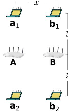
Fig. 7. Topology of two OBSS where each BSS has two clients.
