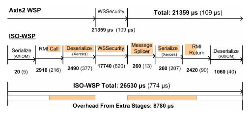
Fig. 5. Comparison of security processing costs for an incoming message. All numbers in microseconds. Numbers in parentheses indicate the 95% confidence interval.
