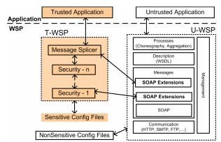
Fig. 3. Architecture of ISO-WSP. Shaded boxes represent Trusted Components. Trusted Components execute in a separate protection domain.
