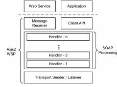
Fig. 1. Web Services Stack. From W3C's WebFigServices Architecture specification [9].Ax
