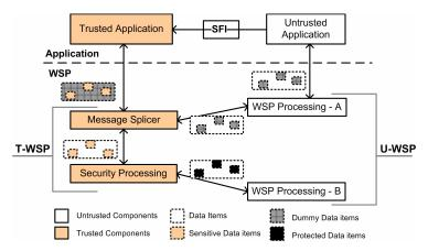
**Fig. 4.** Securing Information Flow in ISO-WSP. The T-WSP replaces security-sensitive data items with protected data items or dummy data items before passing them on to the U-WSP. SFI is discussed in Section 4.
