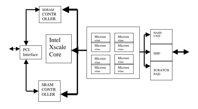
Figure 1. IXP2400 Block Architecture (source, Intel IXA)
