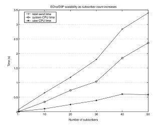
Figure 8. ECho scalability where increasing numbers of clients use the D3P interfaces.
