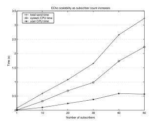
Figure 7. ECho scaleability with no D3P features.
